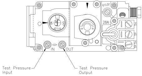
**FIGURE 7. Pressure Test Point Location**
